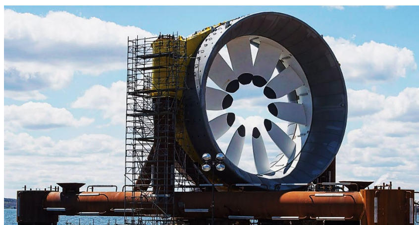
Figure 2. The 2 MW-rated OpenHydro ducted turbine. Adapted from [8], The Canadian Press/Andrew Vaughan, 2016.
