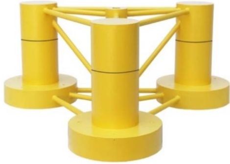
FIGURE 1: OC4 PLATFORM MODEL FOR THE EXPERIMENT [8]
