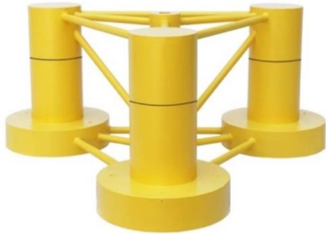
FIGURE 1: OC4 PLATFORM MODEL FOR THE EXPERIMENT [8]
